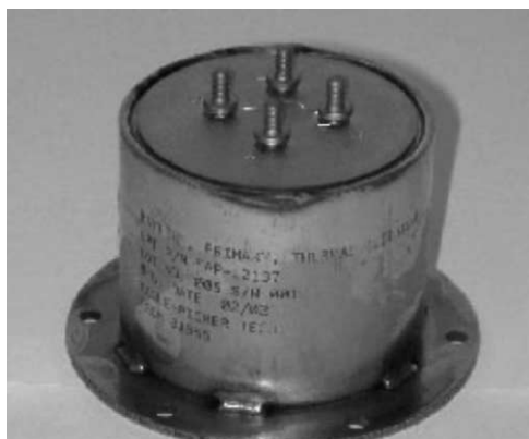
Fig. 8. MER Li-FeS 2 thermal battery, fabricated by Eagle Picher Technologies.
