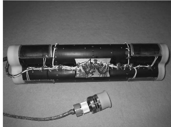
Fig. 7. Lander battery (36 V, 6.8 Ah), one of the five parallel units on MER Lander.
